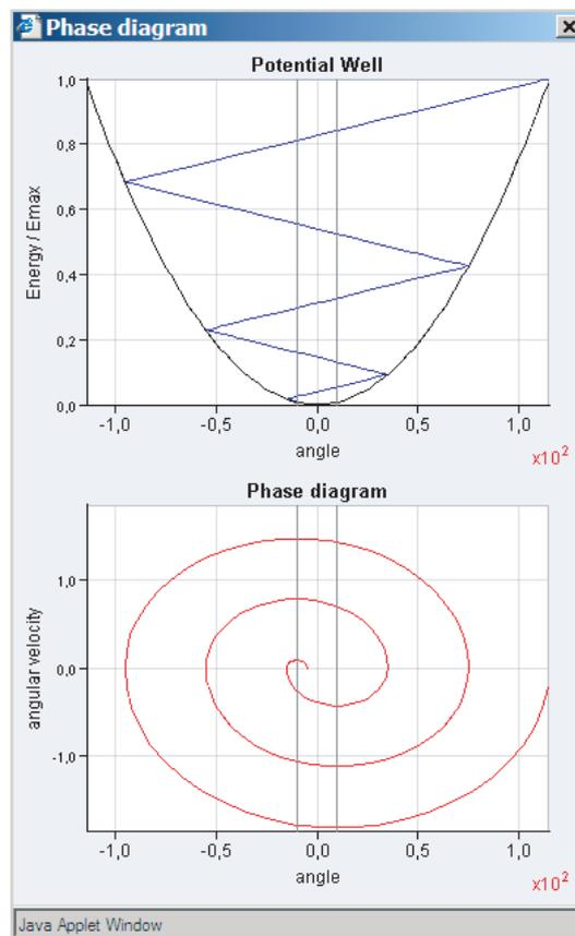
Figure 4: The phase diagram of damping caused by dry friction
