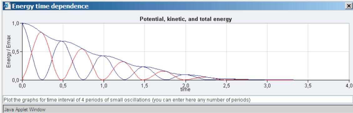
Figure 5: Energy transformations in oscillations damped by dry friction
