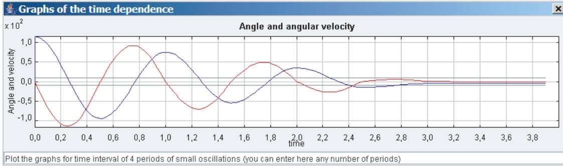
Figure 3: Damping of oscillations caused by dry friction
