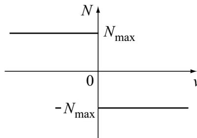
Figure 2: An idealized characteristic of dry friction (*z-characteristic*).
