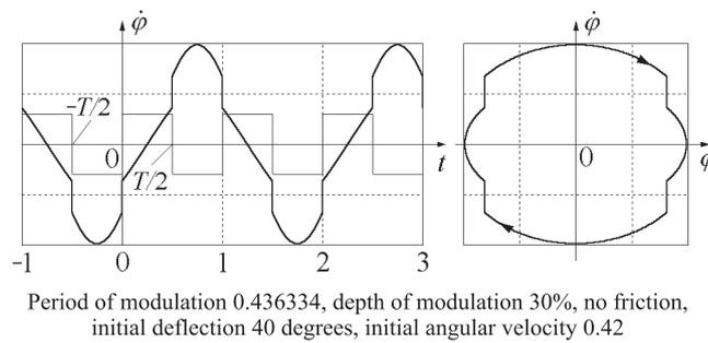
Figure 4: Stationary parametric oscillations at the lower boundary of the principal interval of instability near ( $T = T_{\text{av}}/2$ ).
