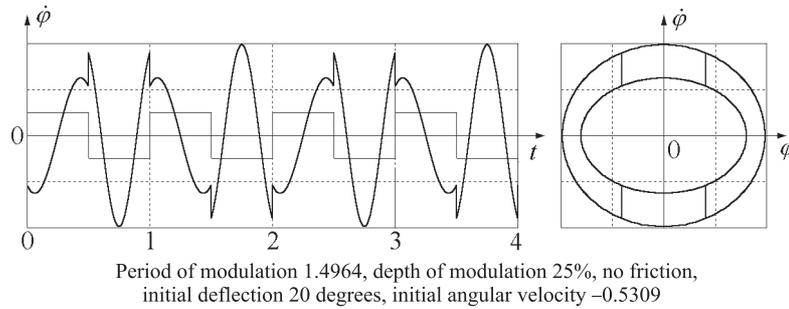
Figure 6: Stationary parametric oscillations at one of the boundaries of the interval of instability near  $T = 3T_{av}/2$ .
