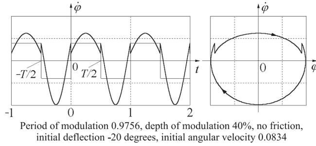
Figure 9: Stationary parametric oscillations at the other boundary of the interval of instability of the second order (near  $T = T_{av} \approx T_0$ ).
