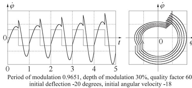
Figure 7: The graph of the angular velocity and the phase trajectory of oscillations corresponding to parametric resonance of the second order ( $T = T_{av}$ ).
