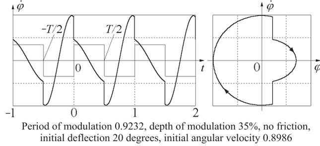
Figure 8: Stationary parametric oscillations at one of the boundaries of the interval of instability of the second order (near  $T = T_{av} \approx T_0$ ).
