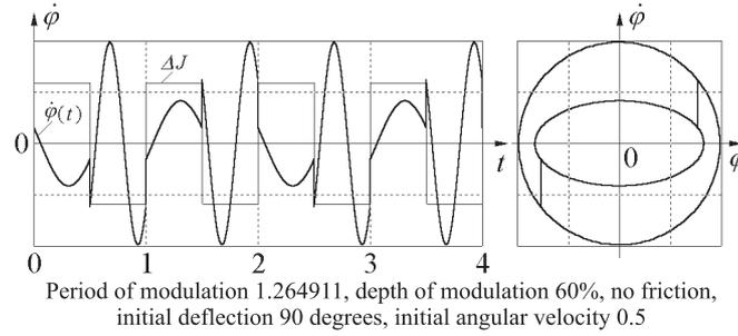
Figure 11: Time-dependent graph of the angular velocity and the phase trajectory for stationary oscillations at the intersection of both boundaries of the third interval.
