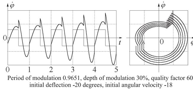
Figure 7: The graph of the angular velocity and the phase trajectory of oscillations corresponding to parametric resonance of the second order ( $T = T_{\text{av}}$ ).
