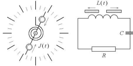
Figure 1: Schematic image of the torsion spring oscillator with a rotor whose moment of inertia is forced to vary periodically (left), and an analogous  $LCR$ -circuit with a coil whose inductance is modulated by moving periodically an iron core in and out of the coil.(right).
