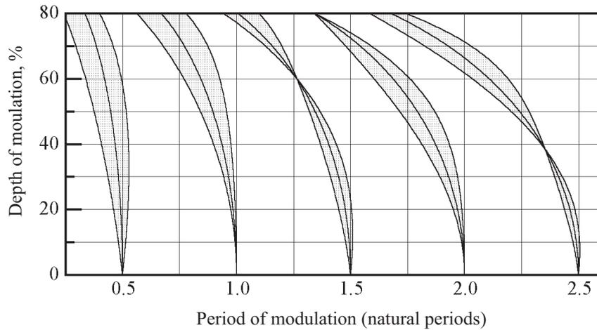
Figure 10: Intervals of the parametric excitation at square-wave modulation of the inertia moment in the absence of friction.
