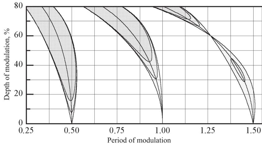
Figure 12: Intervals of parametric excitation at square-wave modulation of the moment of inertia without friction, for  $Q = 20$ , and for  $Q = 10$ .
