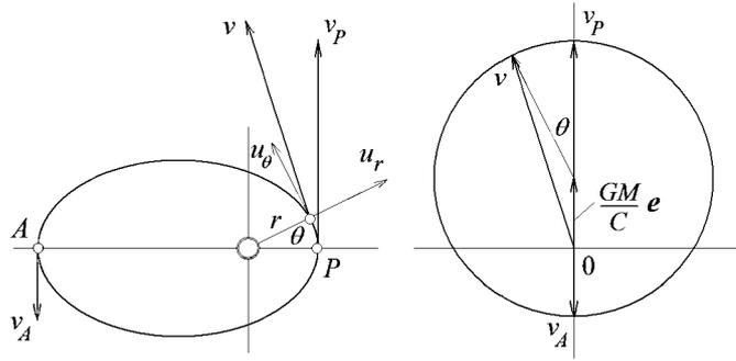
**Figure 1.** Keplerian orbit and the velocity vectors in space (left), and the hodograph of the velocity vector in velocity space (right).
