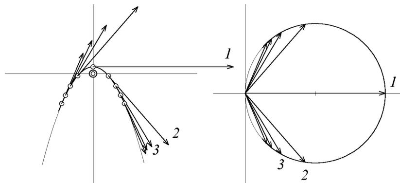
**Figure 2.** Parabolic trajectory of a body in a central gravitational field and the velocity vectors in space (left), and hodograph of the velocity vector in velocity space (right). Identical numbers on the left- and right-hand sides refer to the same instants of time.
