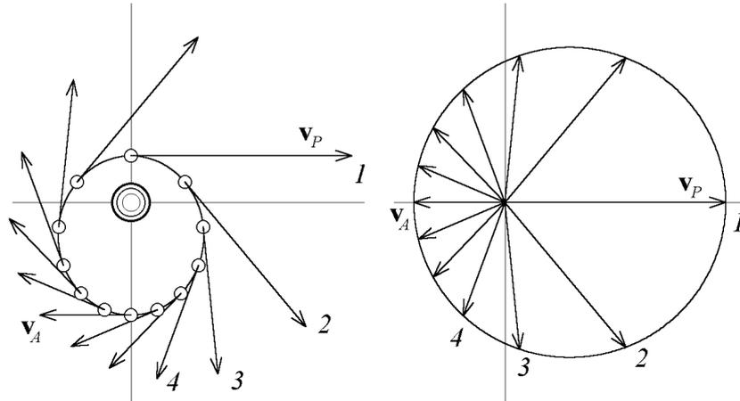
**Figure 1.** Keplerian orbit of a satellite and the velocity vectors in space (left), and hodograph of the velocity vector in velocity space (right). Identical numbers on the left- and right-hand sides refer to the same instants of time.
