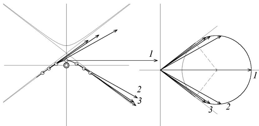
**Figure 3.** Hyperbolic trajectory of a body in a central gravitational field and the velocity vectors in space (left), and hodograph of the velocity vector in velocity space (right). Identical numbers on the left- and right-hand sides refer to the same instants of time.
