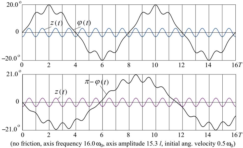
**Figure 3.** The graphs of  $\varphi(t)$  for oscillations of the pendulum about the lower and upper equilibrium positions, respectively, and the graph  $z(t) = -a \cos \omega t$  of the pivot motion. The graphs are obtained by a numerical integration of the exact differential equation (12) for the momentary angular deflection.
