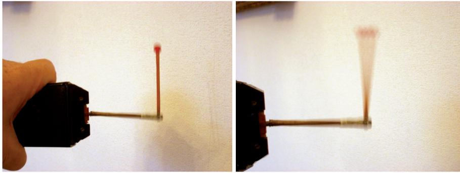
**Figure 1.** Demonstration of dynamic stabilization of the inverted pendulum.
