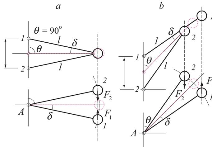
**Figure 2.** The forces of inertia  $F_1$  and  $F_2$  exerted on the pendulum in the noninertial reference frame at the extreme positions 1 and 2 of the oscillating axis  $A$ .
