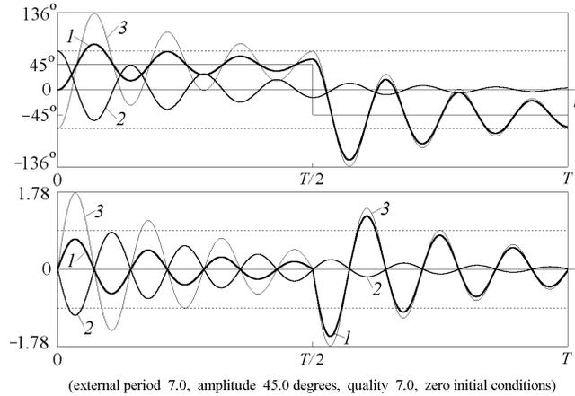
**Figure 6.** Graphs of the angular position (upper part) and velocity (lower part) showing the decomposition of the transient (curve 1) onto the damping natural oscillations (curve 2) and the periodic steady-state oscillations (curve 3).
