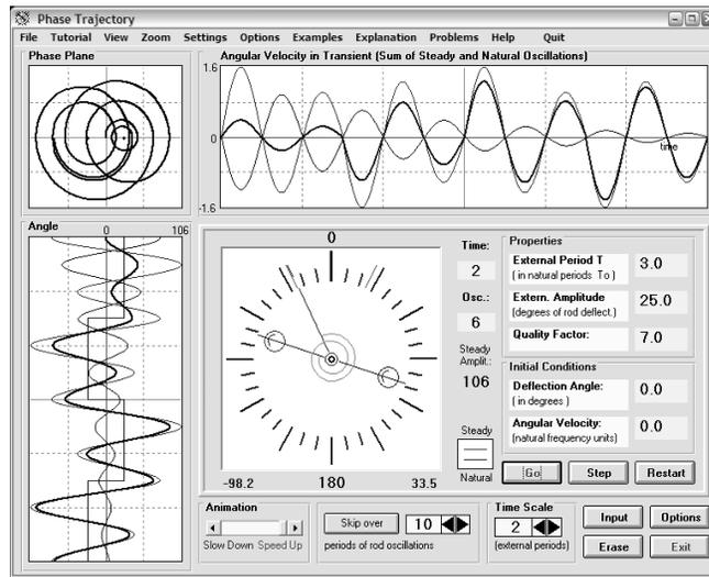
**Figure 5.** Graphs of the time dependence of the position angle and of the angular velocity, together with the phase diagram, for the transient process of excitation from equilibrium for resonance occurring at  $T = 3T_0$ .
