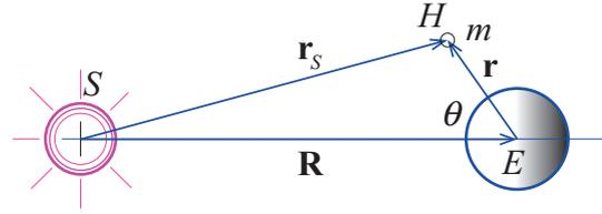
**Figure 3.** For the calculation of the tidal force at an arbitrary point  $H(r, \theta)$  near the earth
