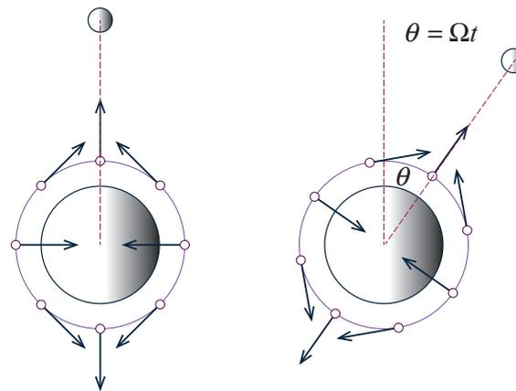
**Figure 5.** The quadrupole configuration of tide-generating forces, rotating as a whole in accordance with the changing apparent position of the moon
